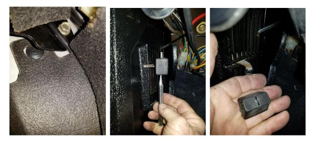
Step 3, Remove the sill cover and the windlace around the door opening perimeter.
