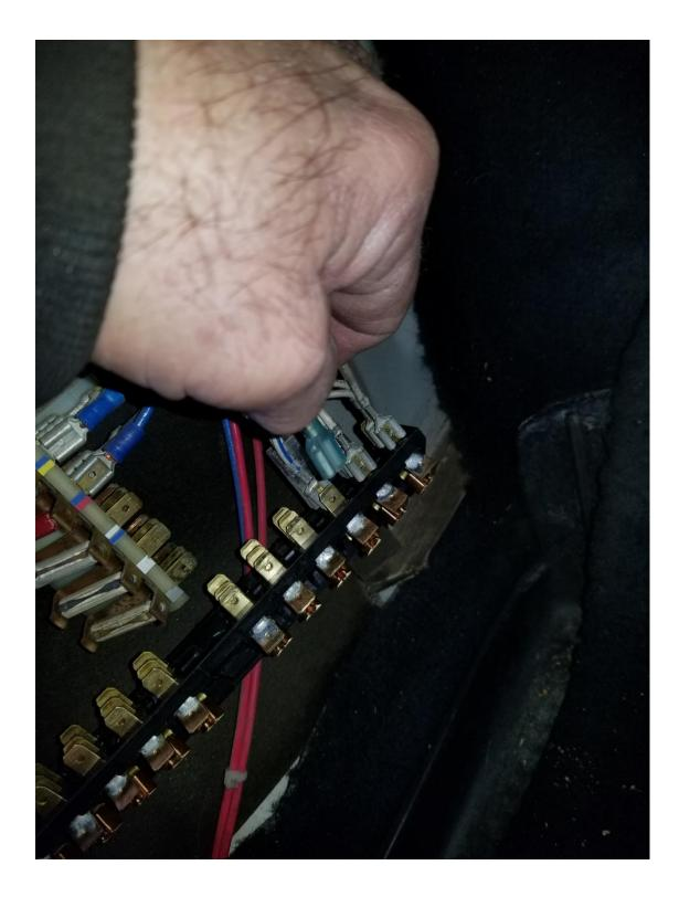
You may want to use a needle nose pliers to help remove/install the terminals. It will give you leverage. Make sure connectors remain tight!
