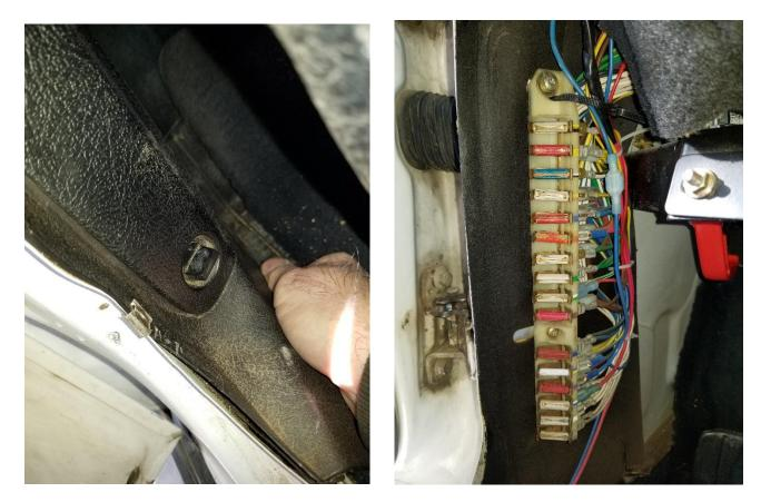
Step 5, unscrew the old fuse panel from the bulkhead and snip any and all cable ties.
