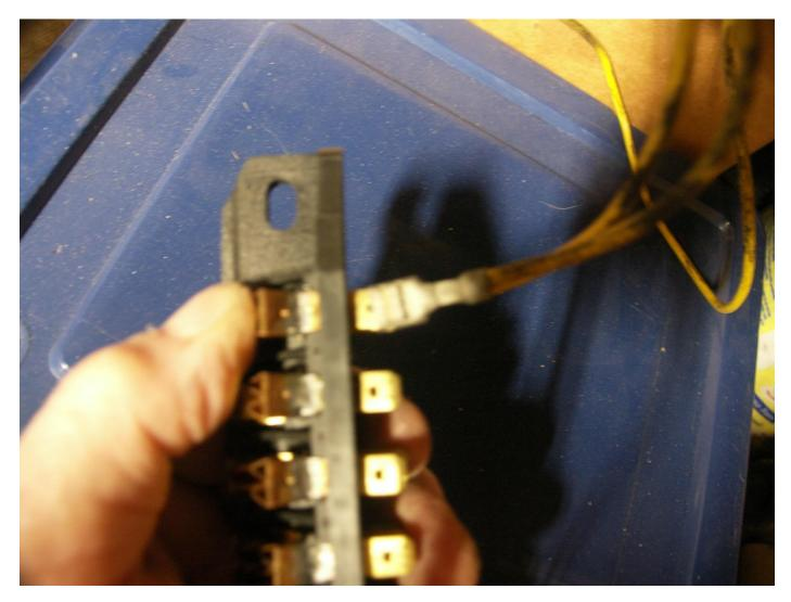
If you find that any female spade from your harness is very loose, crimp it down to tighten it. If it will not crimp tight, it may be cracked. Replace it. Likewise, don't crimp it too tight, or it will not slide onto the panel's connector. If you force it on without supporting the fuse socket, the socket may release from the base. Simply push it back in. Take care not to bend it, as it may snap or crack a solder joint if flexed bent too aggressively.
