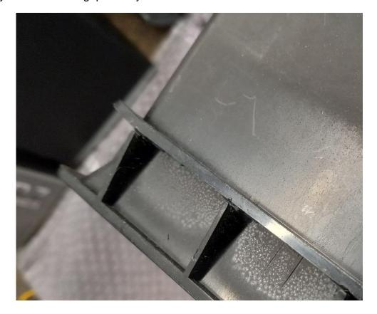
With all the fins cut and separated from the rear housing, remove the entire bezel/window assembly, and set the housing aside. The window has, all around its perimeter, "teeth". These raised tabs are how the window is bonded to the bezel. You'll see these bonds on the bezel perimeter.
