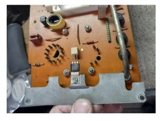
Remove the grounding plate and regulator.
