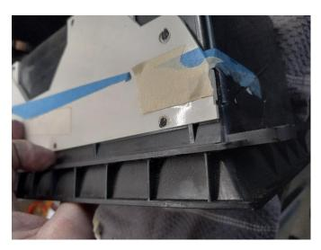
These fins must be cut away from the rear housing for the bezel to be removed, and to gain access to the old window. Using a single edged razor blade, and great care, slice the back of each of the fins to separate them from the rear housing. Cut the fins as perfectly flush to the rear housing's surface as possible. Always take great caution when using razor blades as tools. Here, you can see the gaps cut by the blade.
