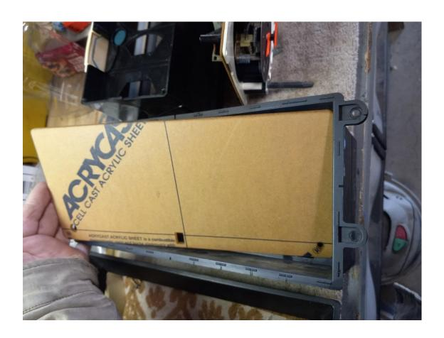
Carefully fit the window down into the rear housing, with the holes in the DEEPEST part. Make sure it seats toward the BOTTOM of the housing. The window has been sized vertically to compensate for the angles, and if there is a slight gap, it needs to be at the TOP of the cluster once assembled.
