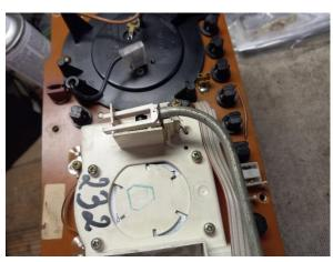
Remove the tube from the speedo housing.
