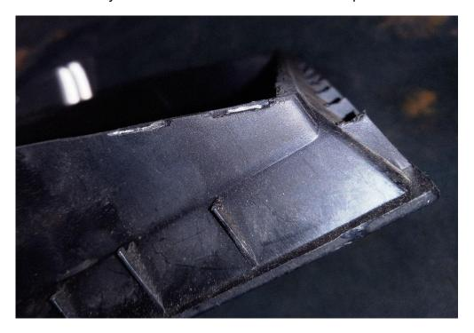
It isn't necessary to do the bottom edge, as that "turns" the other way. If you are using a large belt sander, it allows you to flatten the entire perimeter and remove any damage from grinding out the window tabs. Don't overdo it! The idea is to maintain the "height" of the bezel assembly, as measured at the sides. If you take off too much, the fins will contact the rear housing at assembly time, before you clamp the new window in place.
