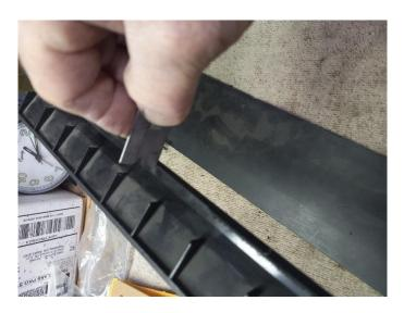
Once you have cleaned all the edges of the bezel, and created a good, smooth surface, with no scrap or threads to dangle in your "view", you are ready to assemble the housing.
