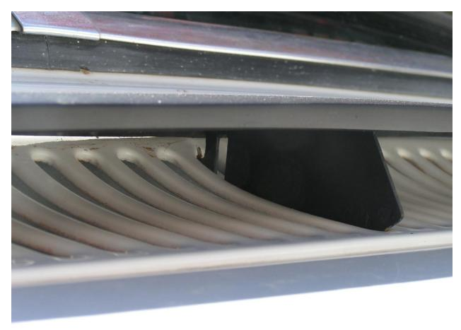
With the center pylon located, drop the anchor blocks through their slots and tighten the screws down. You may need to hold the blocks steady with a screwdriver until they contact the underside of the cowl. Don't over-tighten! If you tighten the screws too much you will deform the snow cap or possibly crack the fiberglass. They are of very heavy construction, but once cracked, they will eventually break.
