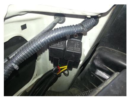
Aforementioned holes not there? Later cars don't have them. Self-drilling sheet metal screws will do the trick. Pay attention to where you drill! Check the other side first.
