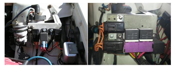
Picture on the left is very tidy, includes a relay for fog lamps. Picture on the right only for fuse holder location, as the relay pack is from an earlier version of the harness. Picture 3, below, from a customer's installation. Extensions for power wires are included.
