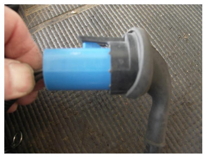
On the passenger side, you will, once again, have an unused plug for both E-code and 9004 harnesses. Since it cannot be removed, we recommend sealing it. A broom handle holder works perfectly for this. Available at hardware stores, or McMaster.com
