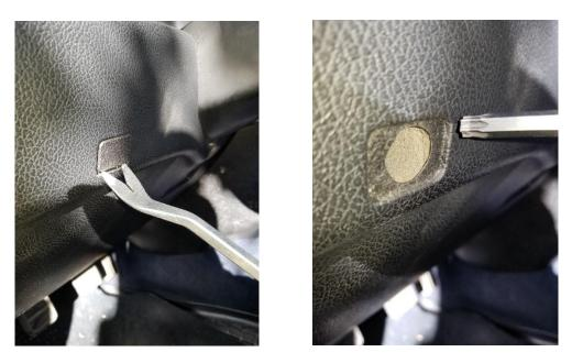
Step 2, regardless of year, the kick panel is held in by a single, snap in fastener, way up under the dash, near the top of the panel. Remove it. A trim tool is handy for this. Early cars will have the foot well vent on the kick panel. Remove the pedal pad by pushing out the pin, then pull off the pad.
