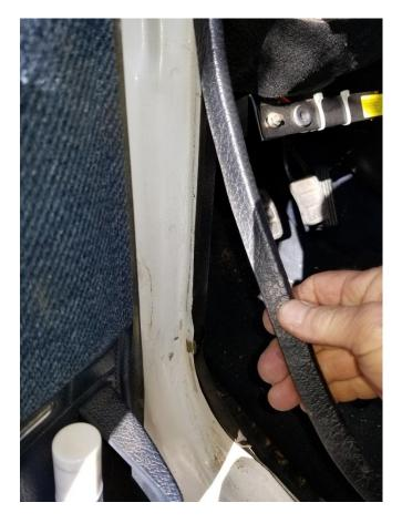
Step 4, remove the kick panel. This will expose the wiring harness and the entire fuse panel.
