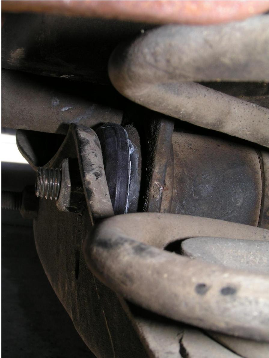
Here in the desert, where rust is not found, even in the dictionary, a few scratches don't matter much. You will undoubtedly have done some damage to the undercoating and paint of the suspension during this process. I highly recommend cleaning up and re-spraying any exposed metal with paint or undercoating spray, including the fasteners. Try and keep paint off the edges of the bushings.
