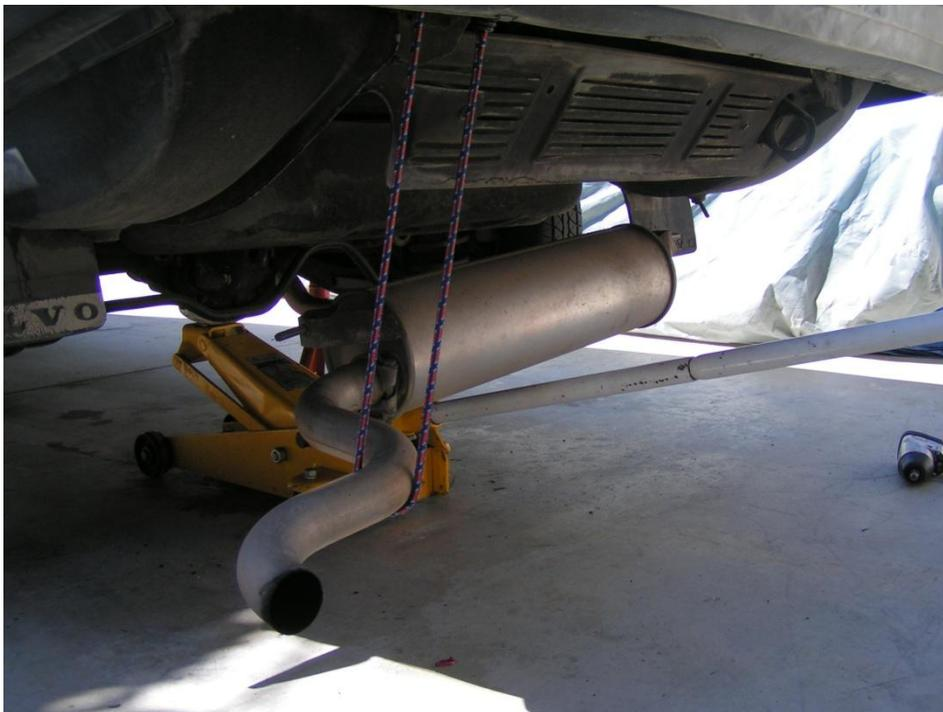
Note how this allows clearance under the axle. Don't leave the muffler dangling without support, you will strain and possibly damage the pipes, and you need to be able to maneuver under the assembly. A bungee cord works well to support the muffler.
