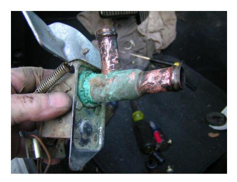
With the heater valve pulled down, remove the capillary tube assembly from the heater box. You will need to pull out the oval rubber grommet too. Here you can see the capillary tube assembly exiting the bottom of the blower motor scroll housing.
