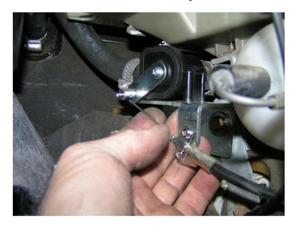
Adjust the wire in the swivel and also the cable in the attachment clamp so that when the heater control lever is off, the valve is fully closed—arm in the up position. You must use almost all the length of the cable to assure the heater control lever on the dashboard moves the valve's arm all the way to "closed". If the valve stays open, your air conditioning will not function correctly.
