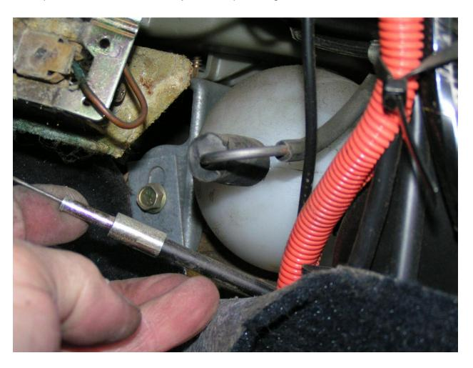
Grasp the old valve firmly and pull the top bracket out of the back of the heater box.
