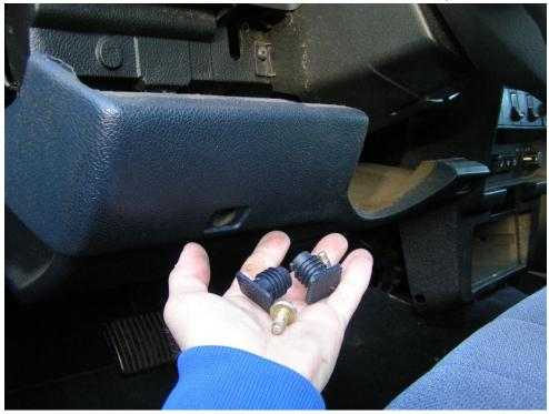
The two screws are Torx fasteners and may be very tight. Once removed you can lower and remove the bolster.
