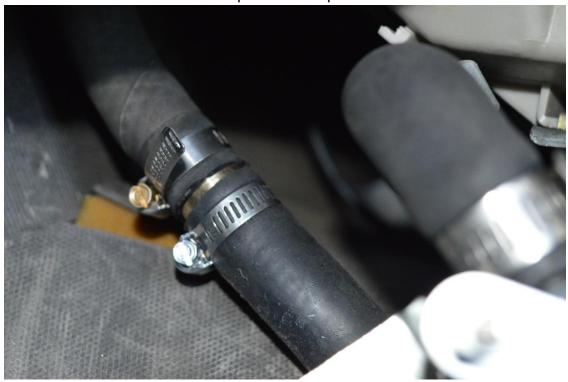
Push the valve back into place against the heater box support where you removed the bolt earlier. Note position of the inlet hose under the outlet hose. Note how the outlet hose's clamp is positioned to clear the actuator arm.
