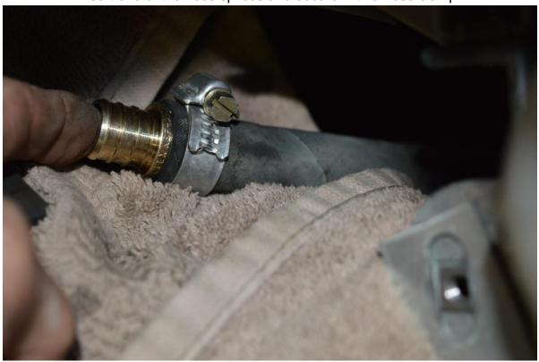
Attach the small elbow hose. The long end goes on the splice.
