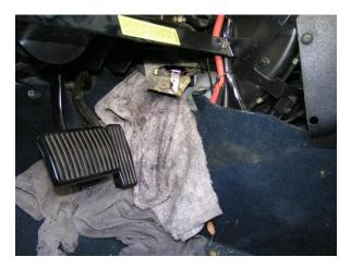
A 1/4" ratchet and 9/32" socket will make removal of the old hose clamps easier if they are original Volvo clamps. Loosen both hose clamps.
