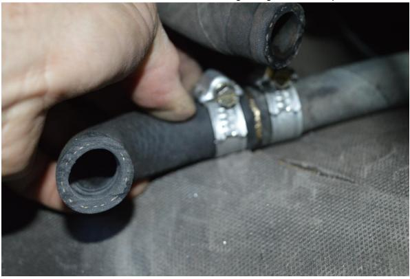
Attach the right angle hose to the arrowed side of the valve (outlet). Note that the hose is pointing slightly upward. That's so it will clear the next hose which you see here already attached to the valve (inlet). Note the orientation.
