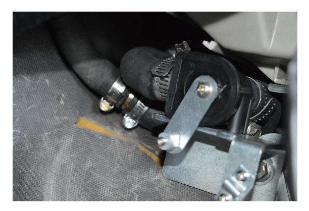
The valve is supplied with a high strength 6mm bolt and nut, two plain washers and one lock washer. Occasionally the captive nut on the vertical brace will be missing. The nut supplied can be used to replace it. If the captive nut is in place, the longer bolt, one plain and one lock washer are all that is needed to attach the valve bracket to the brace. A ratcheting box wrench is a great help here. Start the bolt by hand.
