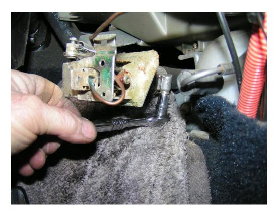
The hoses will be stuck tightly to the valve! Be careful. If you tear them, they will have to be replaced. Work a small screwdriver under the edges of the hoses to help loosen them. The old valve will likely be somewhat corroded, depending on how much humidity has been present. This one was not too bad—a desert car.
