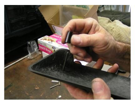
Step three, thread an anchor bar onto the screw.
