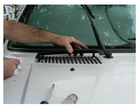
Using the flat head screwdriver to keep the anchor straight, tighten the screws until the anchor is just beginning to contact the underside of the cowl.
