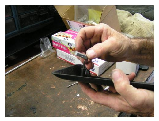
Repeat the process for the other side of the cap. You are now ready to install it on the car. You will need a Philips head and a flat head screwdriver. The flat head is just to reach in and adjust your anchor and screw. Slip the two anchor bars through the second slots from the end of the cowl vent as shown.
